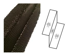
For constructions requiring structural beams to bear relatively higher and different types of loads while resisting delamination, Biteam has pioneered now the Combination Architecture Z-Stringers.
